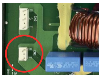
Noise filter power connection
