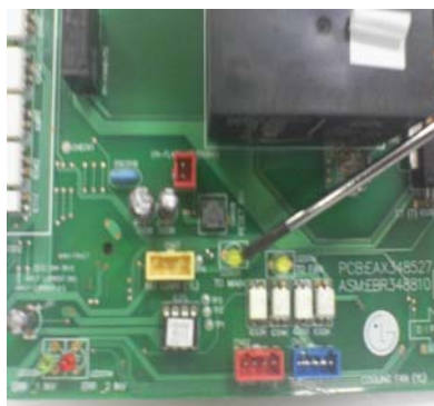
communication connector & LED in inverter compressor PCB
