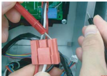
Measuring insulation resistance between fan terminal & chassis
