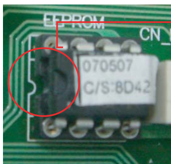
Inverter EEPROM insertion direction
