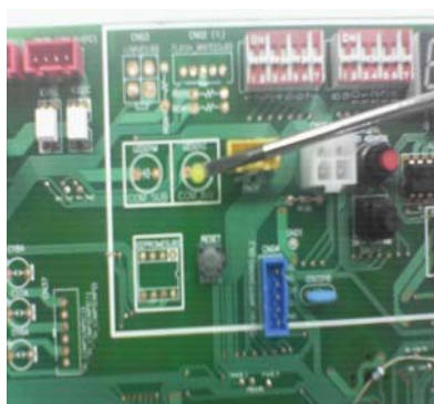
communication connector & LED in MAIN PCB
